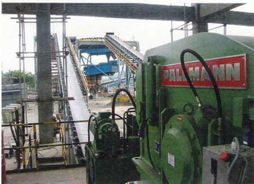
One of two Pallmann chippers at the start of the fiber infeed line
